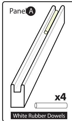
Before starting Step 3 installation, install the white foam dowels into panel A groove. Follow the diagram for the location of the foam dowels. The reason for this installation is to help equally stabilize the C1, C2, and, C3 panels so it does not form a gap.
