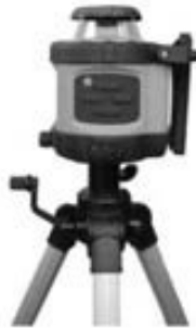
Connect the laser with the tripod using the 5/8" - 11 screw thread
