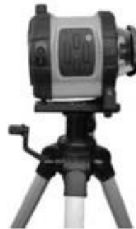
Connect the laser with the tripod using the 5/8" - 11 screw thread
