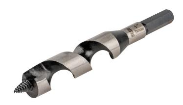
The deep, open-throat design of the Ship Auger bit clears chips for faster, cleaner cuts. The shank is 7/16-Inch hex to fit 1/2-Inch (13 mm) and larger three-jaw chucks. Used for heavy construction and repair work in mines, on docks and bridges as well as electrical work.
