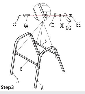
Tighten all screws and Place F on top of it.
