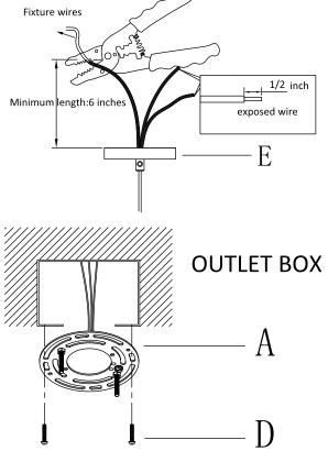
Twist wires together with plastic wire connector (C) until tightly joined.
