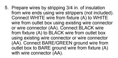
**NOTE:** Screw wire connectors (AA) on in a clockwise direction.
