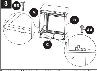
Hand tighten (AA & BB). Do not tighten with wrench (FF), until all bolts
