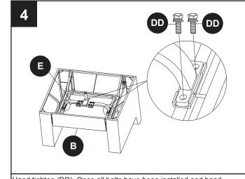
Hand tighten (DD). Once all bolts have been installed and hand tightened, go back and tighten firmly with wrench (EE & FF).
