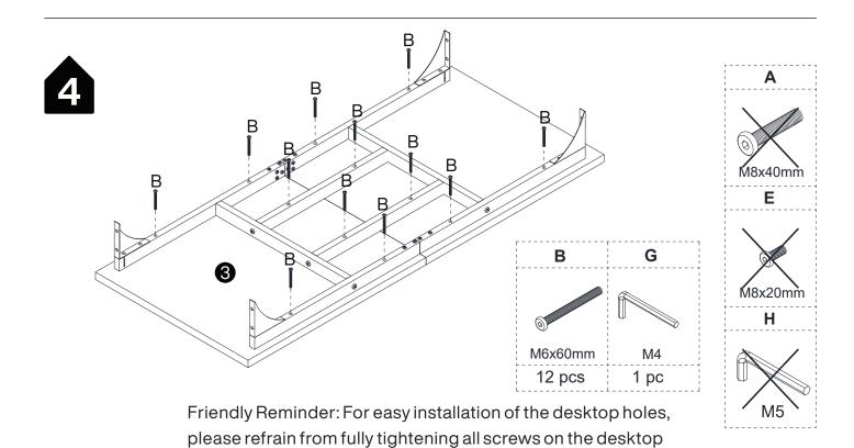
First, screw them halfway in until all screws are attached into the desktop board. Then proceed to tighten all the screws evenly.
