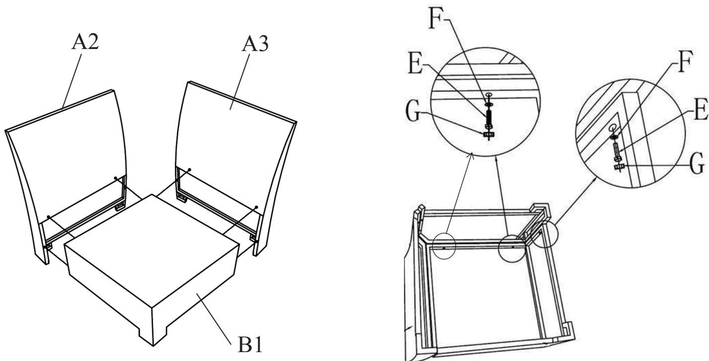
**Step 2** Connect the two back panels by using 2 Connectors (C), 4 short Bolts (D) and 4 Washers (F). Finally put bolt Caps (G) until all parts have been connected and bolts are tightened.
