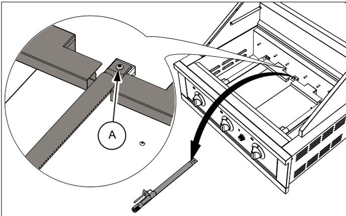
**2** Loosen the screw on the air shutter valve and turn the air shutter valve to change the air opening.
