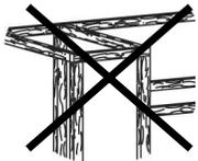
Cabinet frame, cabinet side panels and counter top must be made from non-combustible material.
