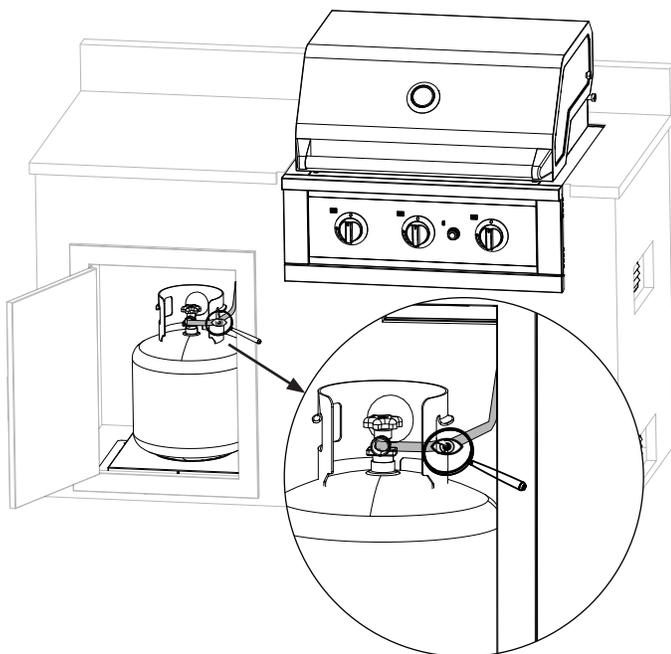
HOSE SHOULD HAVE A SMOOTH SNAKED PATH TO PREVENT KINKS AND PREMATURE FAILURE. PLEASE EXAMINE HOSE AND FITTINGS FOR CRACKS, TEARS, OR WEAR MARKS FROM RUBBING ETC.
