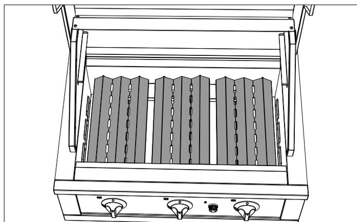
**4** Install the three cooking grates on top of the Flame Tamer Panels as shown.
