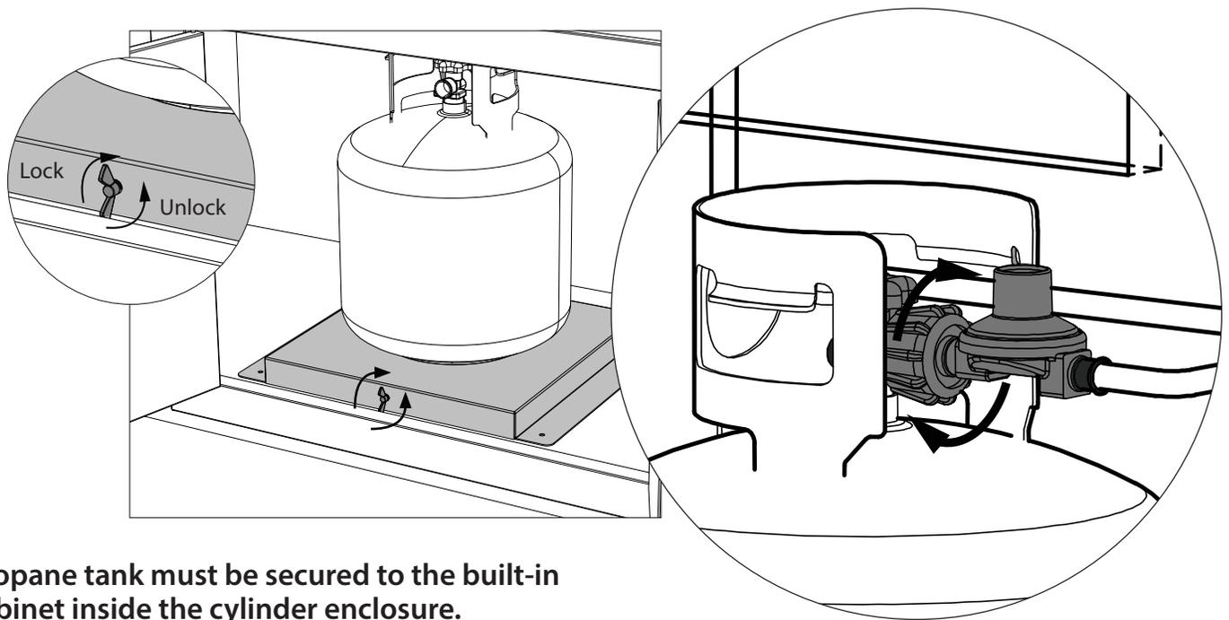
Propane tank must be secured to the built-in cabinet inside the cylinder enclosure.
