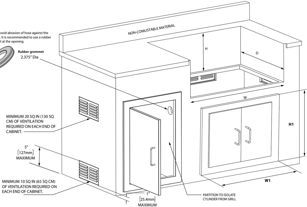
**Note:** The cabinet should not be designed in a way that a spare cylinder can be stored inside the enclosure.
