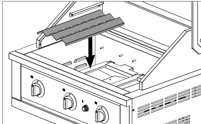
**2** Make sure the Flame Tamer Panel sits properly on the dowel pins as shown below.
