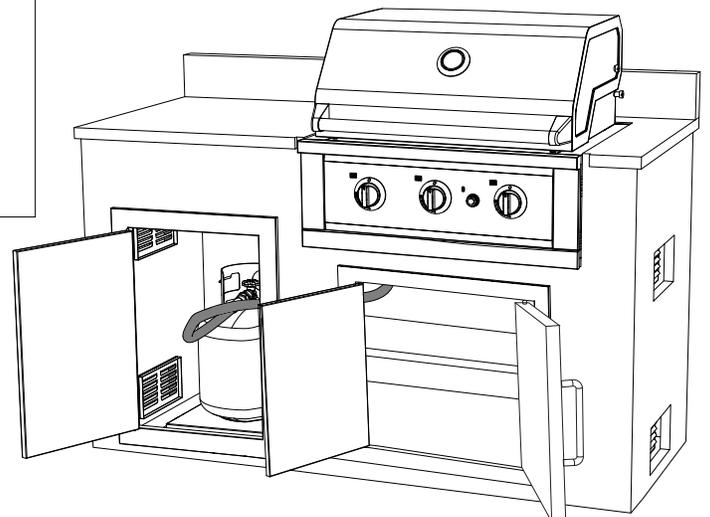
**Propane tank must be secured to the built-in cabinet inside the cylinder enclosure.**
