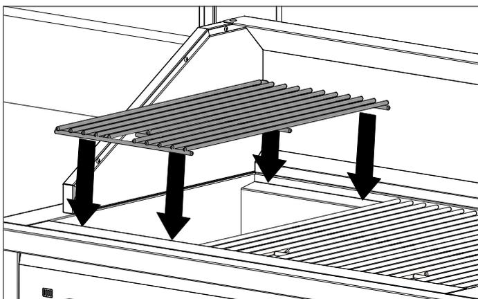
**5** Install the warming rack, by placing it on the provided brackets.
