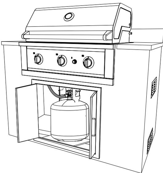
Propane tank must be secured to the built-in cabinet inside the cylinder enclosure.
