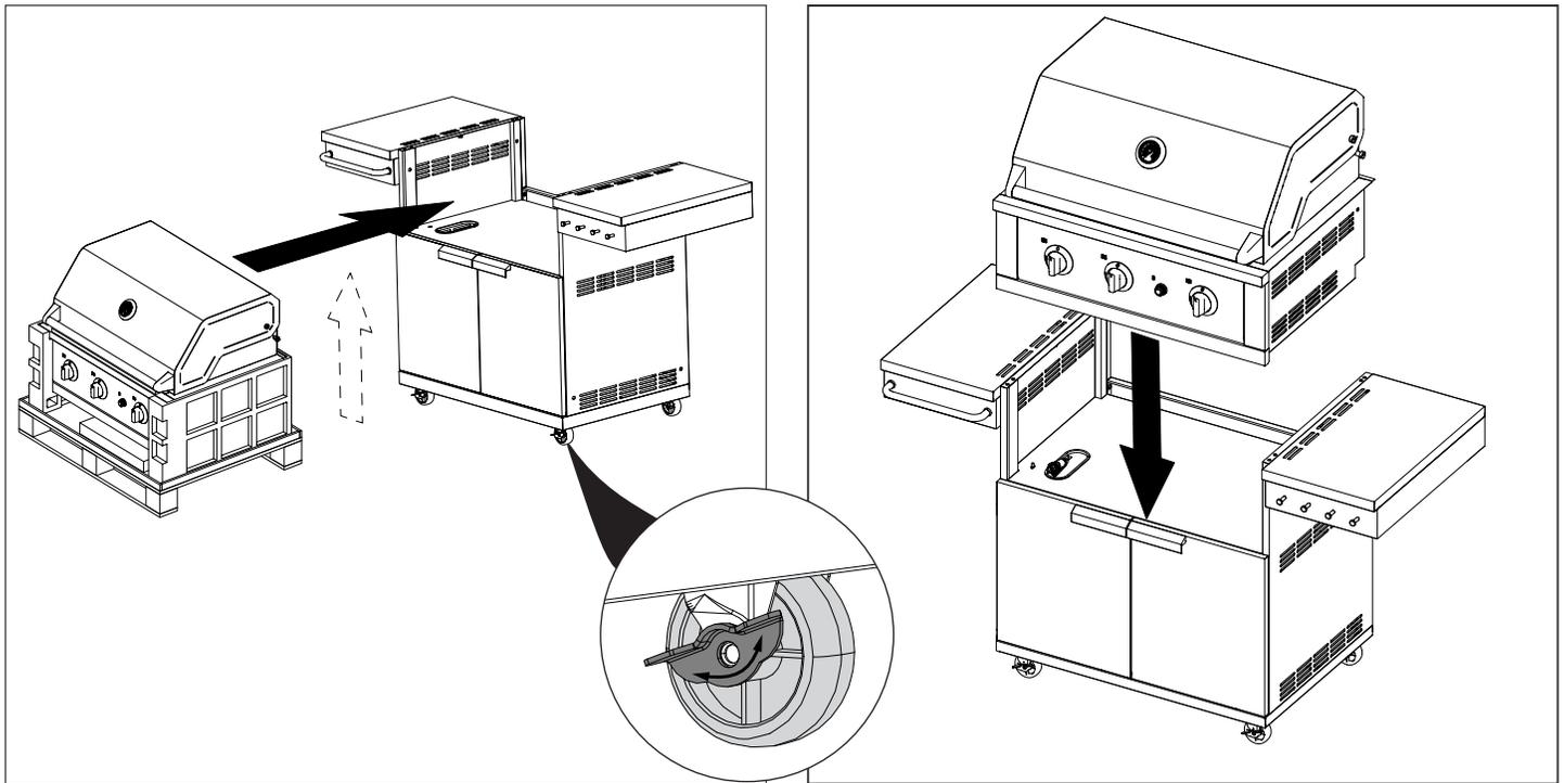
**NOTE:** When you are ready to install the appliance, place it directly onto the Cabinet/ Cart.
