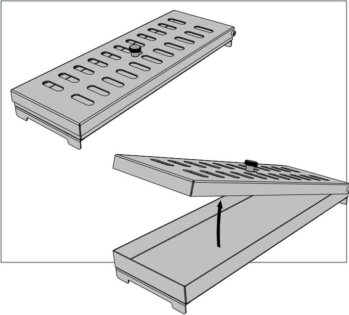
**i** Smoke vents can be adjusted by sliding the knob to control the smoke intensity.
