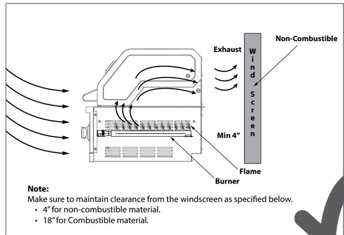
During the high wind conditions, it is best if you don't use your grill. If located in consistently windy area (oceanfront, mountaintop, etc.) a wind break will be required. Always adhere to the specified clearances as defined in the "Installation Manual".
