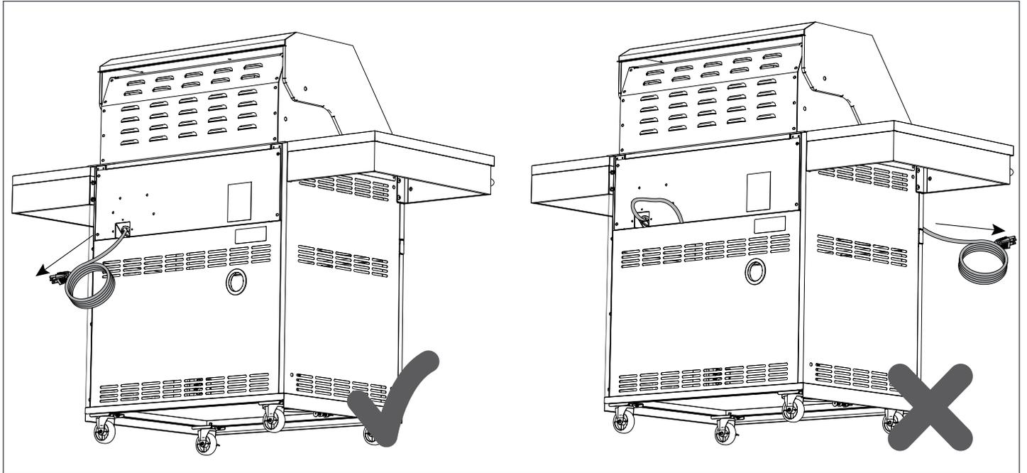
**NOTE:** While connecting the gas hose to the grill, make sure the hose is not bunched up below the grill. (Applicable to Grill Cabinets and Carts both)
