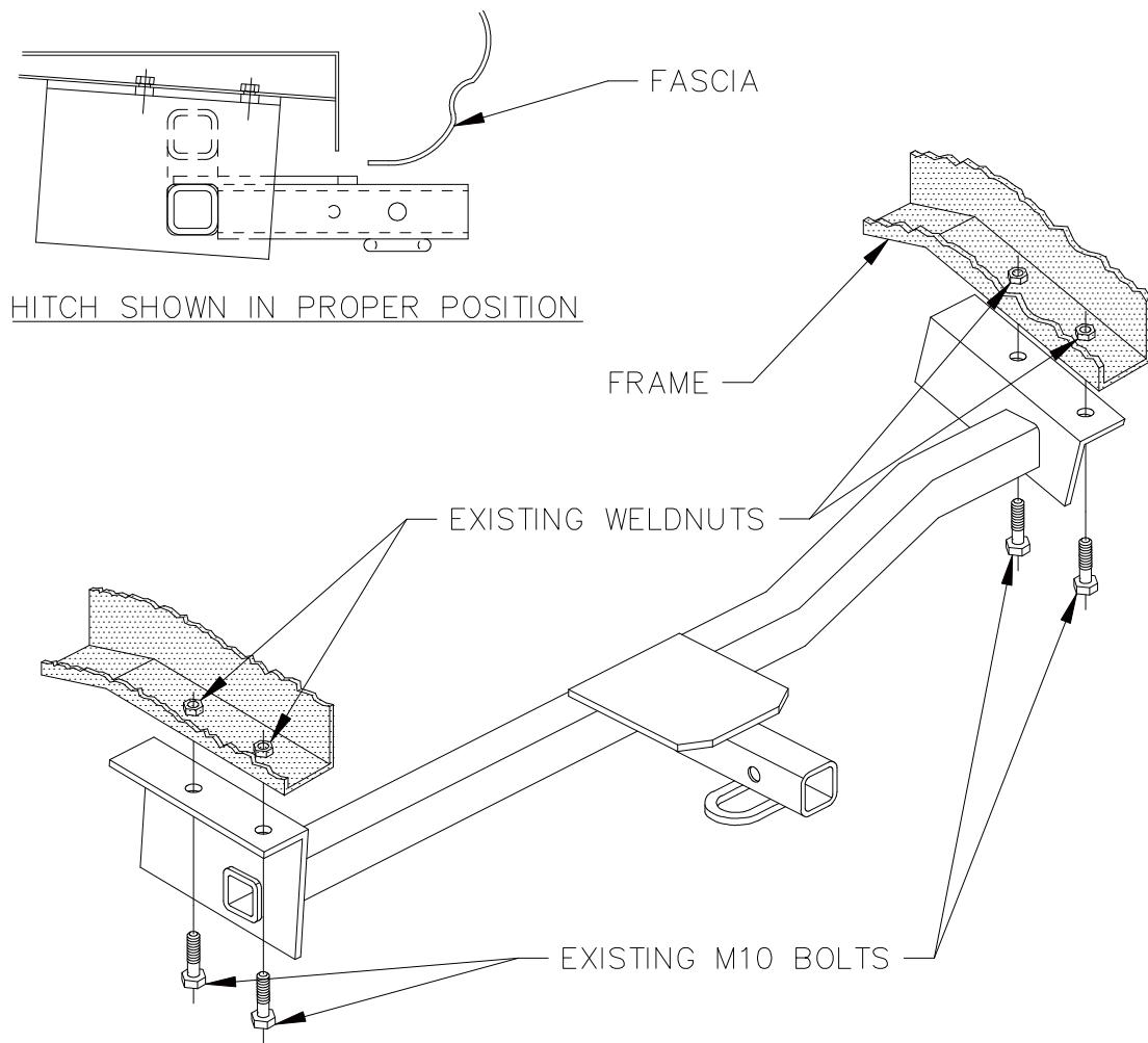
1. REMOVE THE TIE-DOWN BRACKETS FROM EACH SIDE OF THE VEHICLE AND RETURN TO VEHICLE OWNER. RETAIN EXISTING M10 BOLTS TO INSTALL HITCH.
