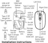
The X9RF2ACMOUSE does not require special drivers and will automatically be recognized by the computer as soon as the dongle is inserted into a USB port. Simply follow the steps below and you are ready to go!
