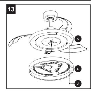
14. Connect the 2-pin connector from the fitter plate (K) to the 2-pin connector from the light kit (L).
