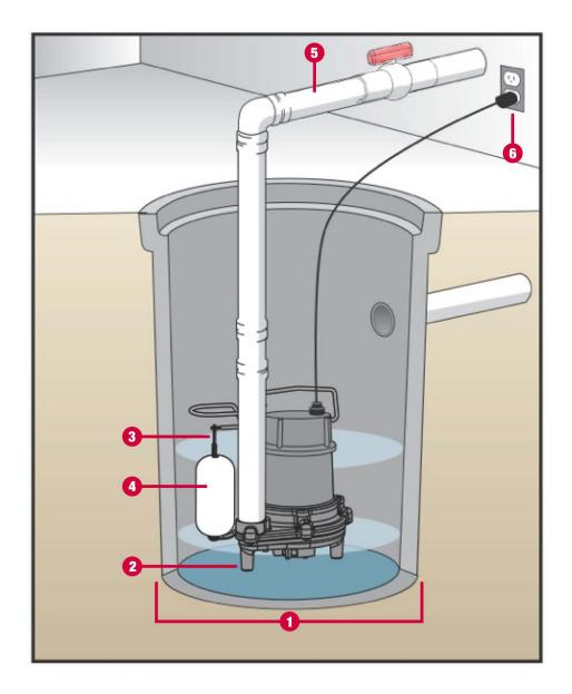
STEP1 Pump must be installed in a suitable basin that is at least 24 inches deep and 11 inches wide for pumps fitted with vertical on/off switches.
