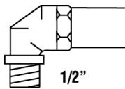
We recommend checking that the appliance is properly set up for the type of gas distributed. The connection to the gas pipes must be made in a workmanlike manner, in compliance with current standards that prescribe the installation of a safety tap at the end of the pipe. The threaded ½" gas connection pipe is located at the rear on the right hand side of the appliance.
