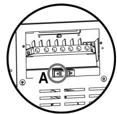
This appliances **is preequipped** at the factory with an electric supply cord set 4 wires type with  $\frac{1}{4}$ " flanged spade terminals (L1, L2, N, Ground) suitable for range use UL/CSA listed type SRDT 2x6AWG + 2x8AWG rated for 125/250 VAC, 50A with plug type NEMA 14-50P; cable length 4'.
