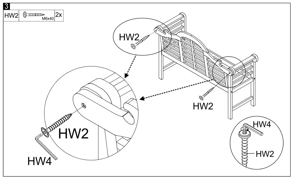
Step 3: Using the Allen screw S (HW2) to fix the Back (A) to chair as shown in the picture by the Allen key (HW4).
