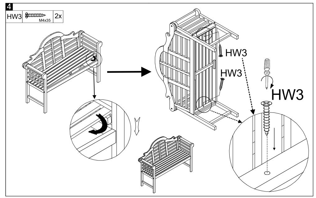
Step 4: Put the Seat (B) to the chair and using the Screw (HW3) to fix the Seat (B) to the chair both sides by the Screw driver before using as shown on the picture .
