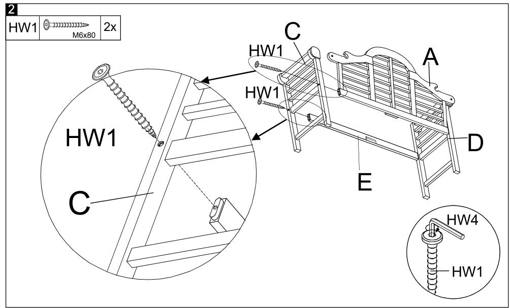
Step 2: Attach the Left side (C) to these parts as shown on the picture .Using the Allen screw (HW1) to fix the Left side (C) as shown on the picture by the Allen key (HW4) .
