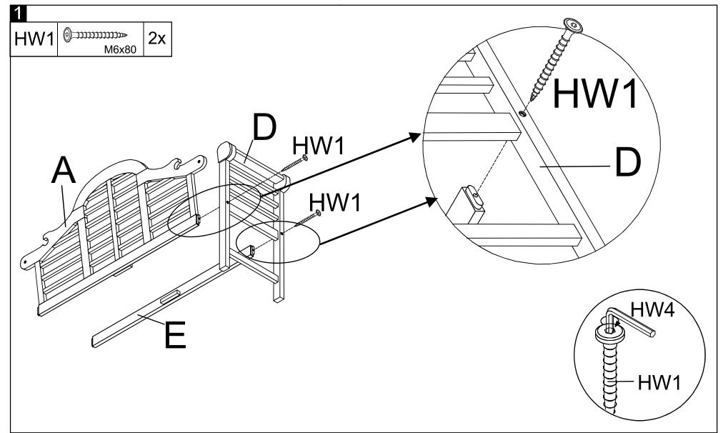
Step 1: Attach the Right side (D), Front Bar (E) to the Back (A) as shown on the picture .Using the Allen screw (HW1) to fix these parts to the Back (A) the Allen key (HW4).
