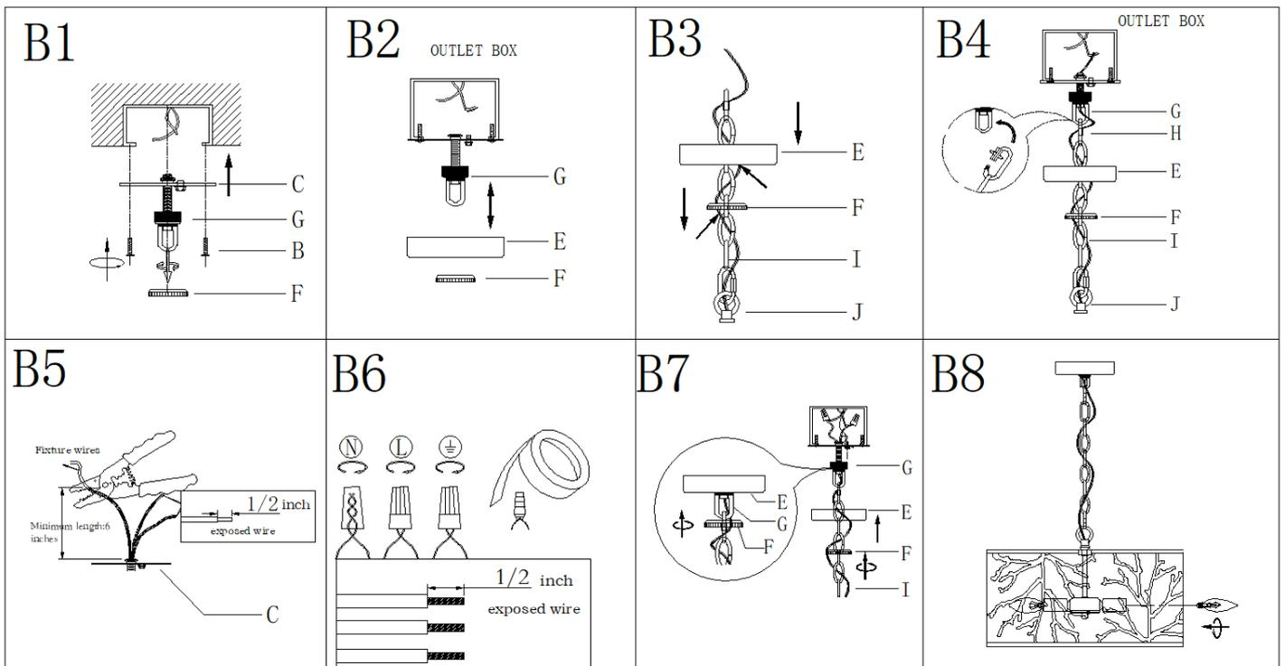
Step B1: Remove the collar ring (F) from collar loop (G). Attach the single bar (C) to the outlet box with mounting screws (B). **Note: the side of single bar marked "GND" must face out.**
