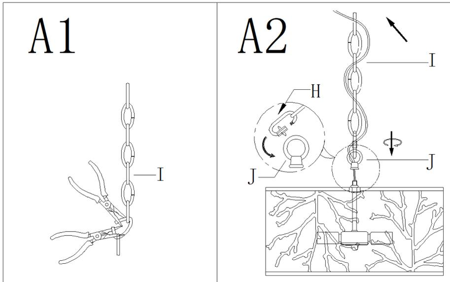
Step A1: By measuring, determine the correct number of links needed for proper hanging height. Using the chain pliers, disconnect and discard the unwanted part.
