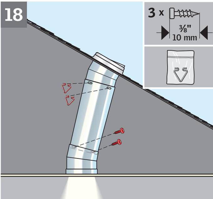
**ENGLISH:** Connect tunnel assembly with the clips supplied. If tunnel section was trimmed or holes do not align, use the screws supplied as necessary.
