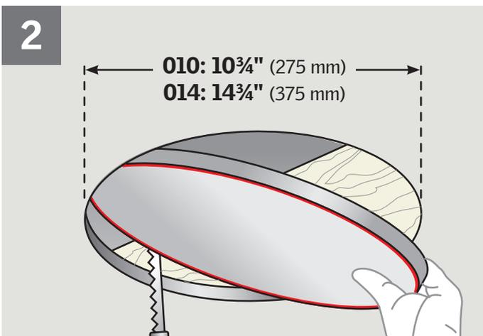
**ENGLISH:** From the inside, locate the nail indicating the center of the sun tunnel in the ceiling, mark circle and cut rough opening in the ceiling as shown.
