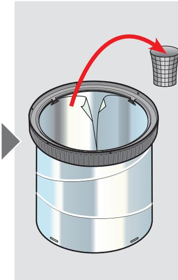
**ENGLISH:** Attach the upper elbow to the pivot ring. Remove protective film from the upper elbow.
