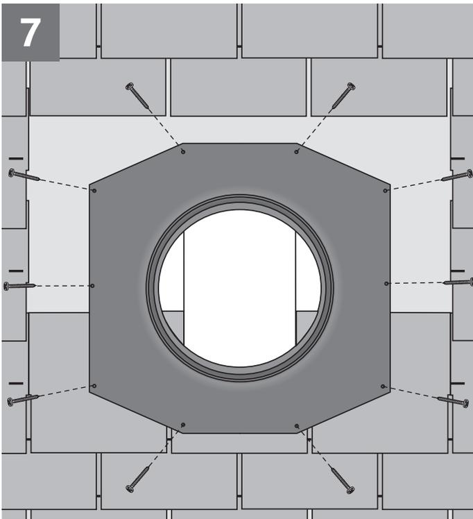
**ENGLISH:** Center the flashing over the rough opening and secure the flange with screws in all the pre-punched holes along the edges.
