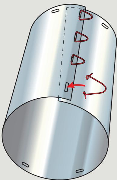
**ENGLISH:** Assemble the rigid tunnel section with tunnel clips provided.
