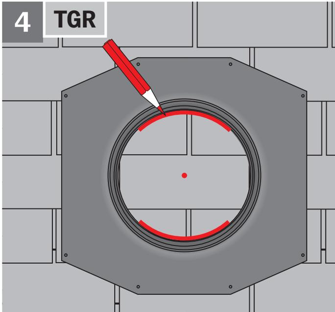
**ENGLISH:** Locate the nail indicating the center of the sun tunnel on the roof and use the flashing to mark top and bottom of the rough opening.
