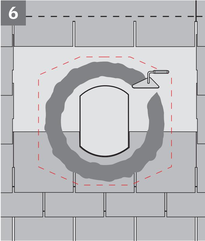
**ENGLISH:** Remove the roofing material around the upper half of the rough opening as indicated and apply mastic around rough opening as shown.
