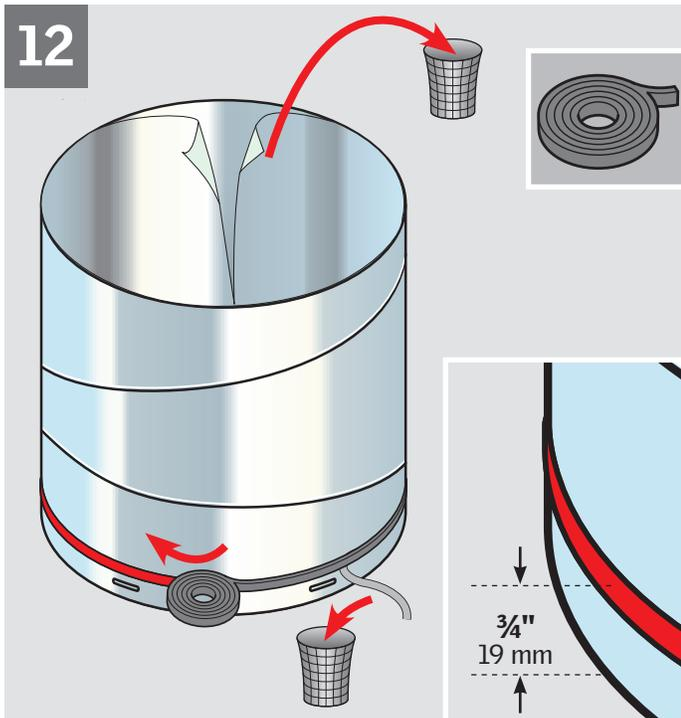
**ENGLISH:** Attach pile gasket to lower elbow as shown. Remove protective film from the lower elbow.
