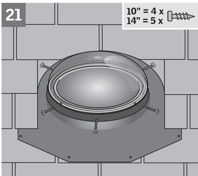
**ENGLISH:** Align holes; install and secure the dome with the  $\frac{3}{4}$ " (19 mm) screws provided. Do not overtighten the screws.
