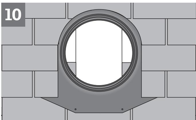
**ENGLISH:** Reinstall roofing material over the flange. Leave a 5/8" (15 mm) channel for water to run off.
