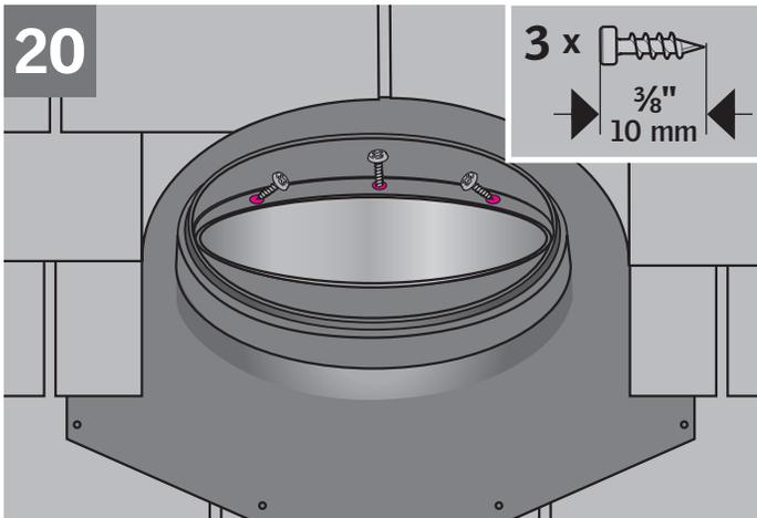
**ENGLISH:** Seat the pivot ring with the tunnel assembly into the flashing. Secure with screws if needed.
