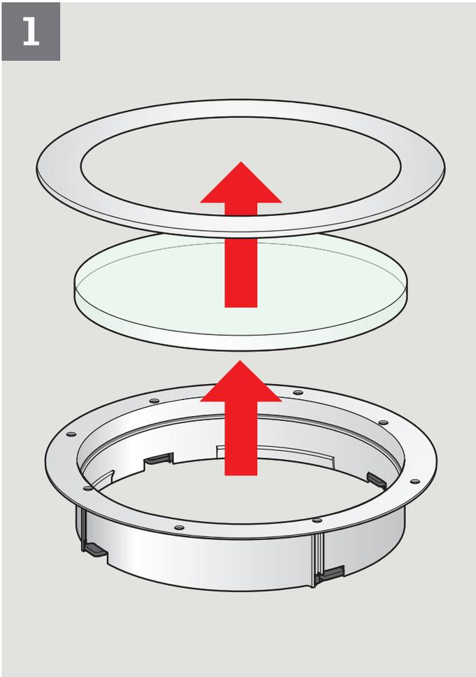
**ENGLISH:** Carefully remove the other parts from the ceiling ring. Rotate trim ring to disengage.
