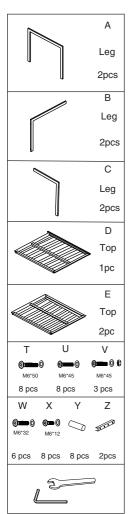
■ Conect the Part A with Part B using connector Part Z and Bolt X as shown in diagram.
