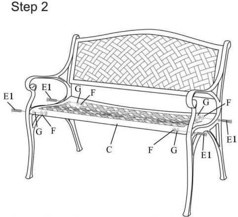
Attach the seat plate (C) to the 2 armrests (A) with 4 bolts (E1) x 4 washers (G) x 4 nuts (F). It's hard to install them by hand, you need to use wrench for the better installation.
