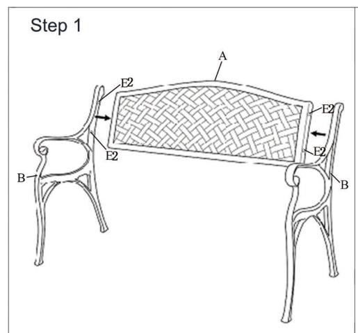
Attach the backrest (A) to the 2 armrests (B) first with 4 bolts (E2).
