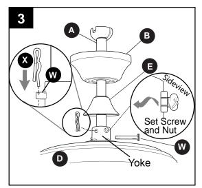
Insert downrod (A) through canopy (B) and yoke cover (E). Then, thread wires from motor housing (D) up through downrod (A).
