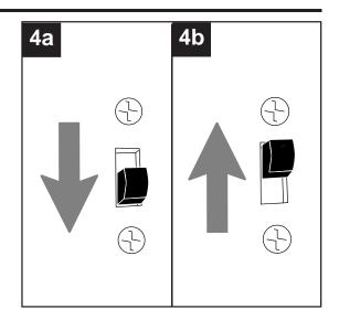
4c. **IMPORTANT**: Reverse switch must be set either *completely UP* or *completely DOWN* for fan to function. If the reverse switch is set in the *middle* position, fan will not operate.
