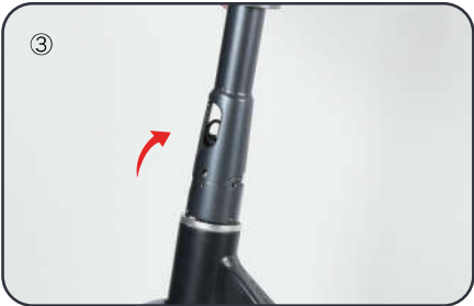
Keep the scooter rod vertical, press and lock the folding handle
