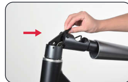
Rotate the folding handle to the snap position to complete the folding.
