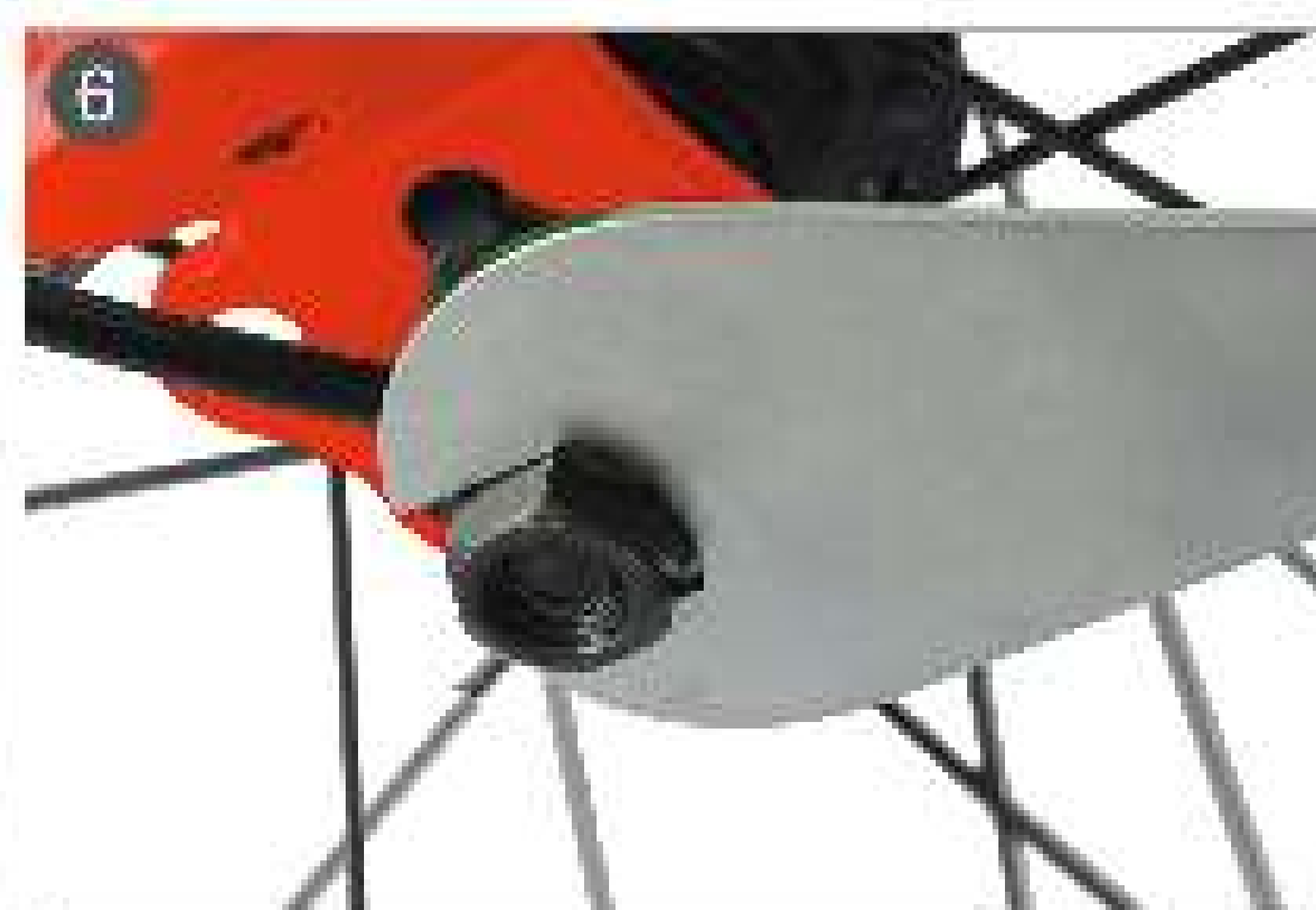
6. Tighten the screw.
