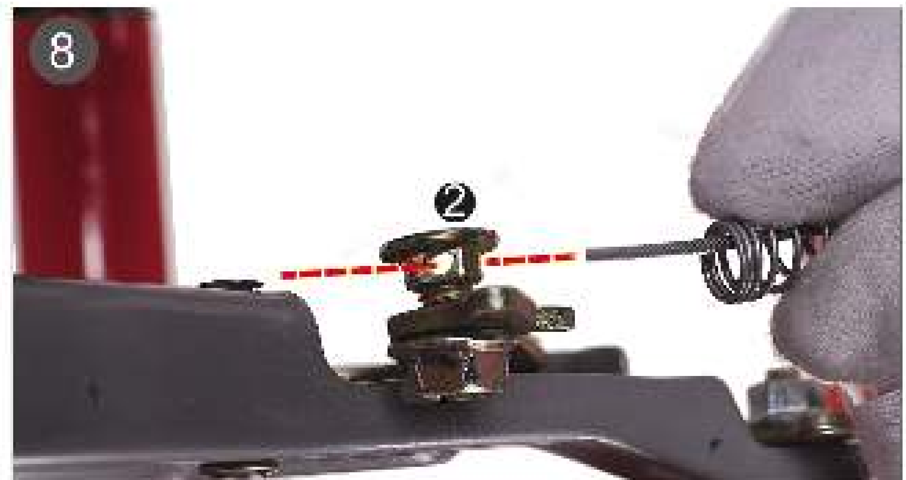
8. Run the wire through hole NO.2.
