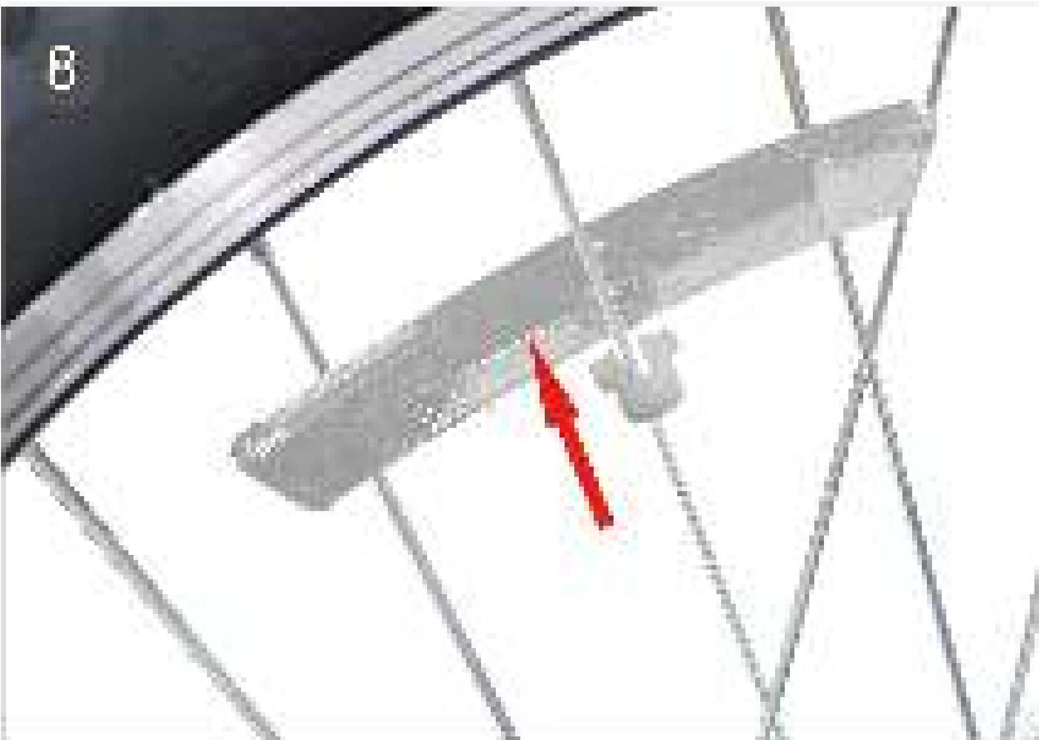
8. Attach the reflectors on the wheel.
