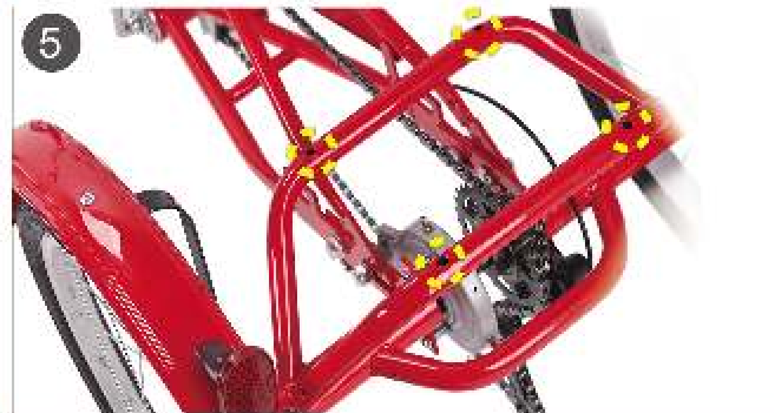
5. Four holes for fixing basket.
