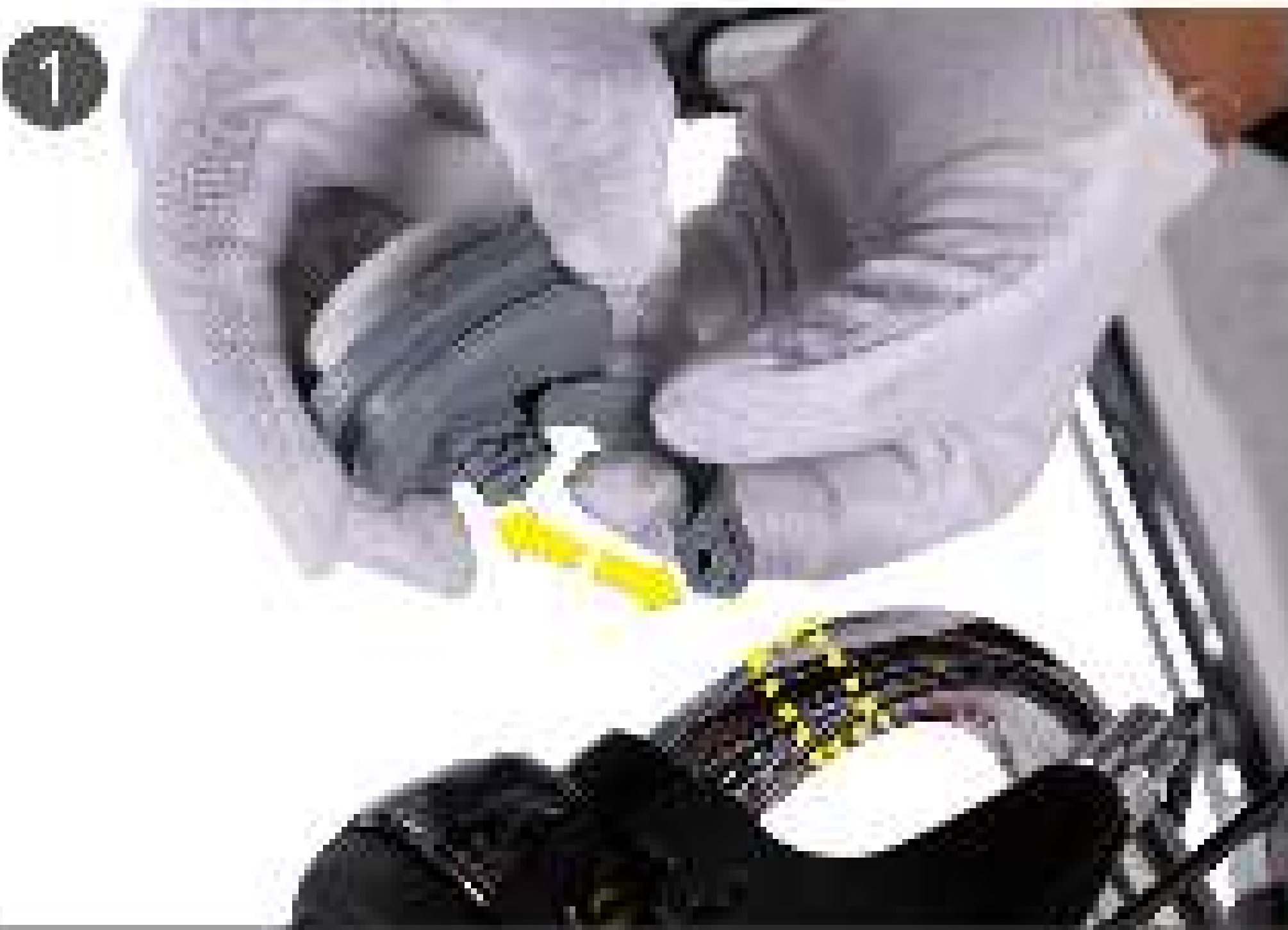
1. Attach the bell on the handlebar.
