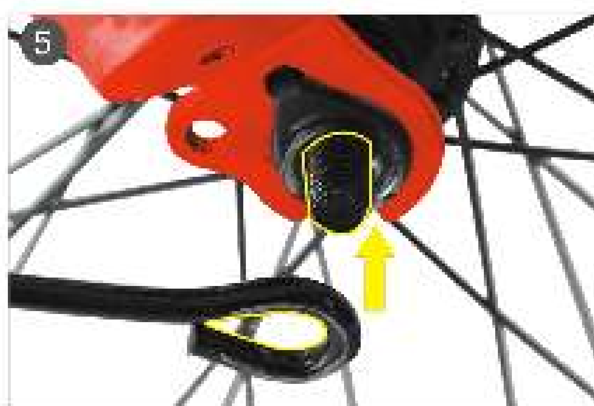
5. Assemble the fender holder.
