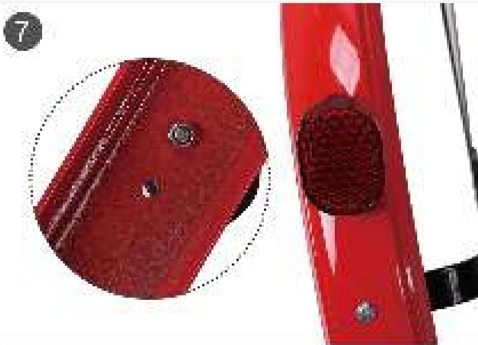
7. Tighten reflector with screw.
