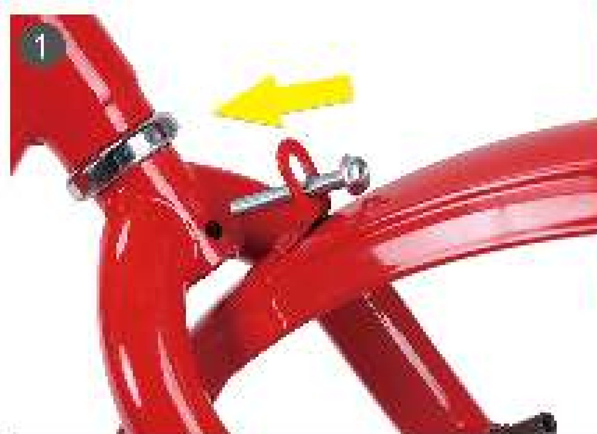
1. Assemble the front fender.
