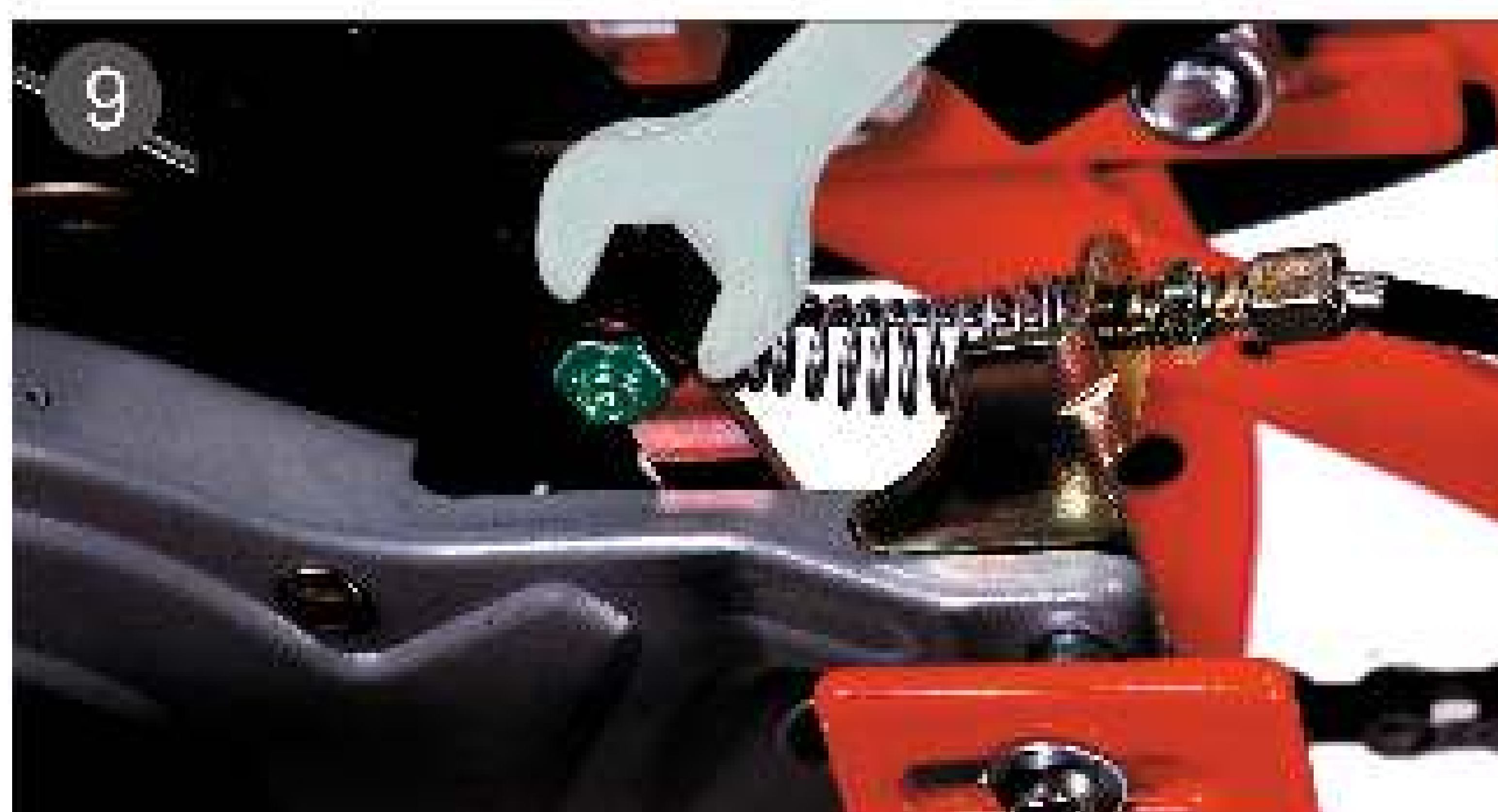
9. Tighten the screw.
