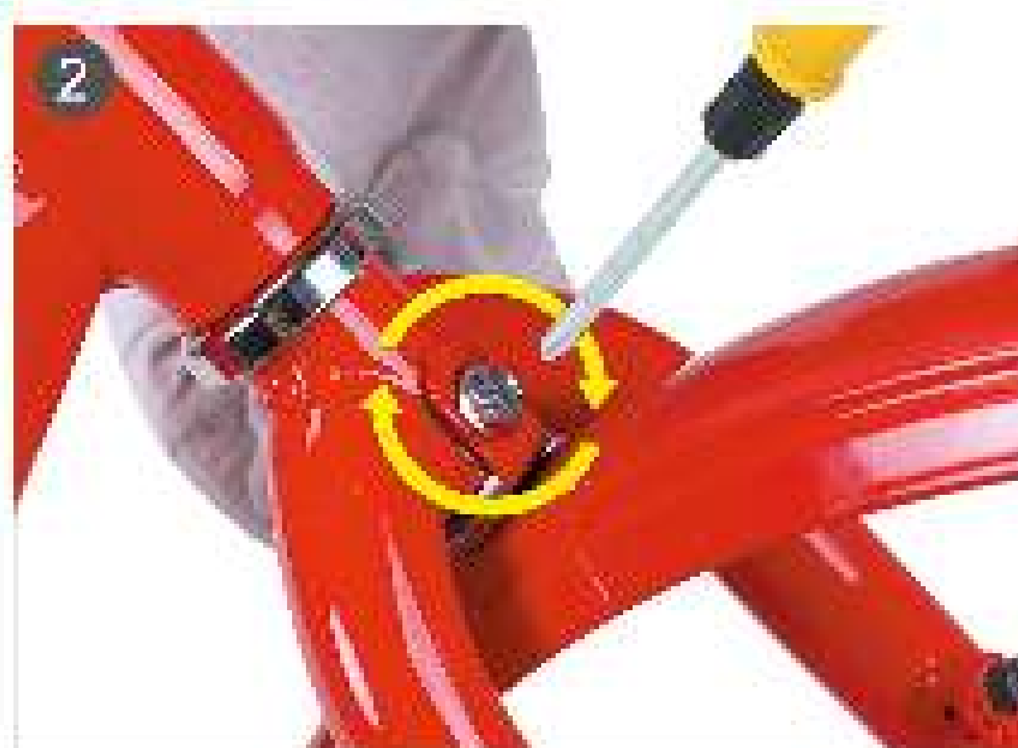
2. Tighten the screw.
