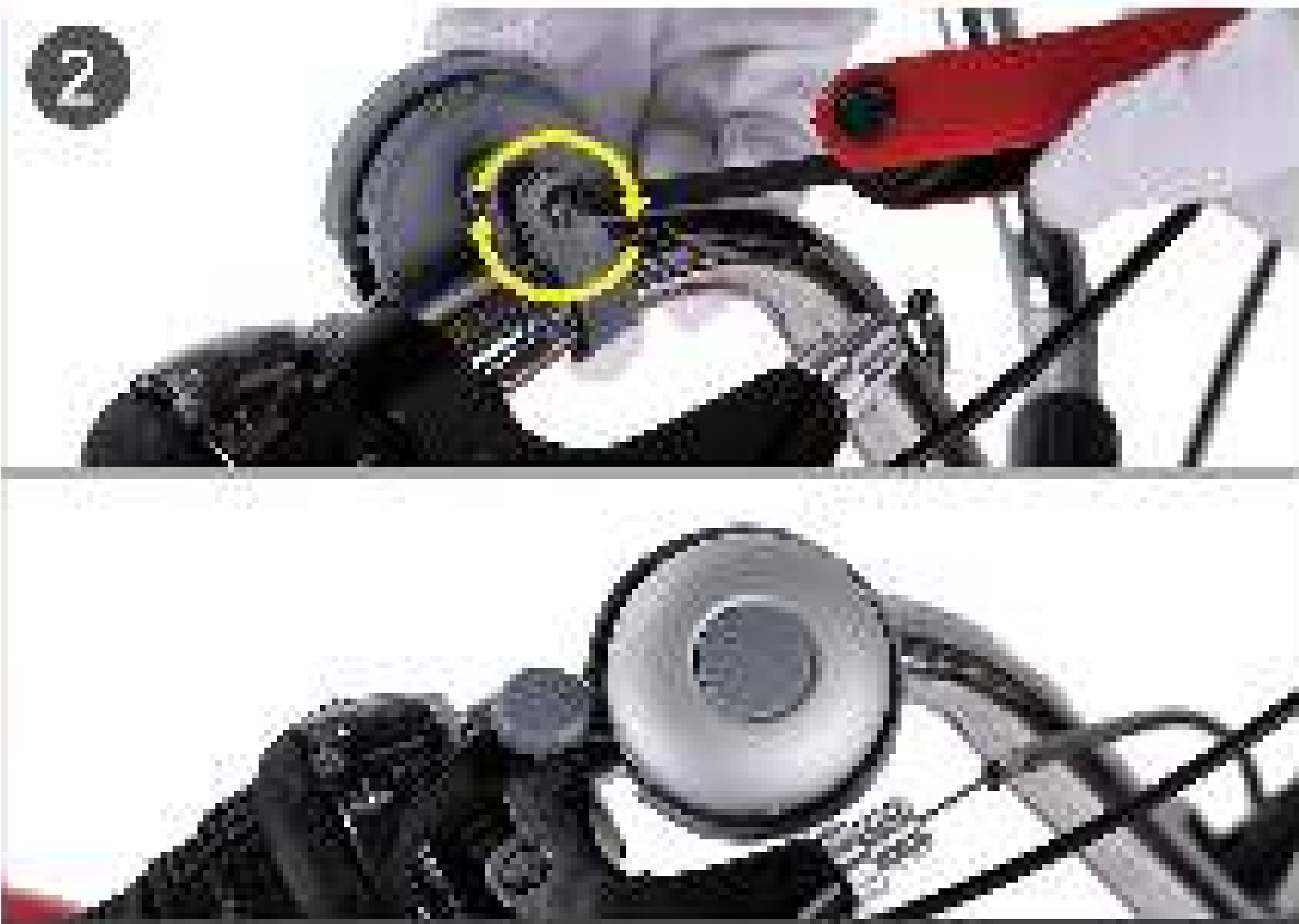
2. Tighten the screw.
