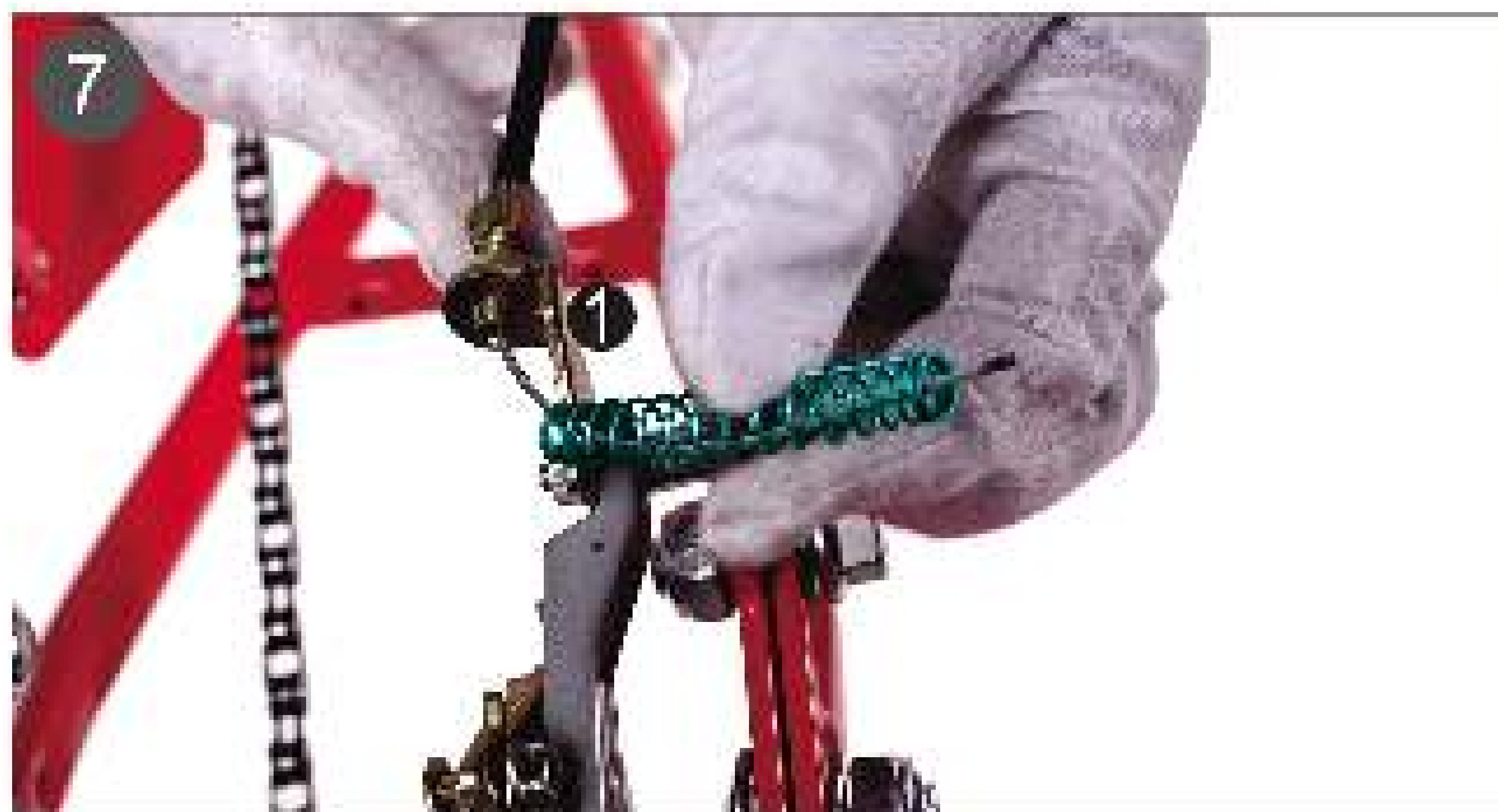
7. Put on the brake spring.
