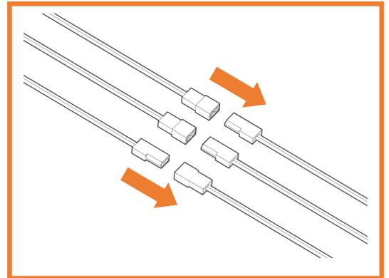
Ensure the cable locks are fully engaged.
