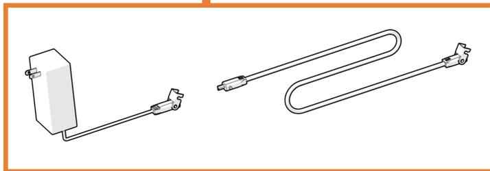
Locate Power Supply pack, connect cables and connect to wall outlet to power unit.
