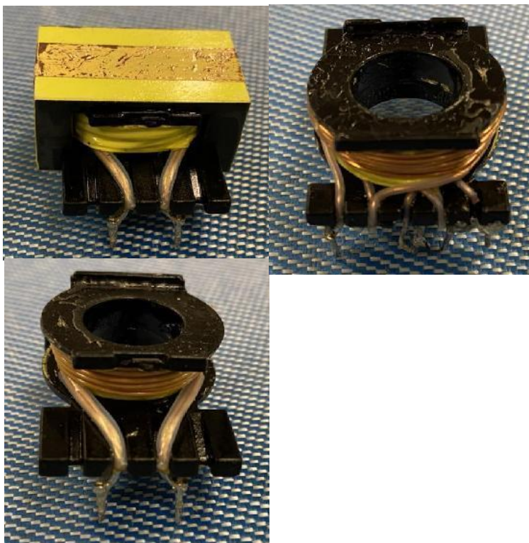
Photo 26 - Internal view of Transformer, model EQ2612
