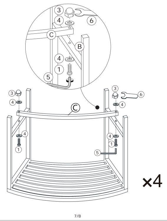
Adjust alignments and NOW TIGNTEN ALL SCREWS with Allen key.
