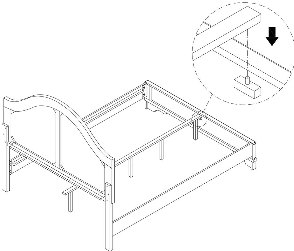
8 Adjust the leveling feet of the legs ⑤ to ensure all slats ④ are leveled and staying at the same level.
