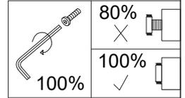
**2** Please completely tighten the bolt D in this step.
