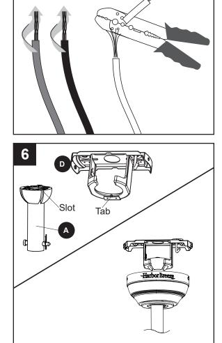
Install the ball end of the downrod (A) into the opening of mounting bracket (D). Align one of the four slots in the ball with the tab in the mounting bracket (D).
