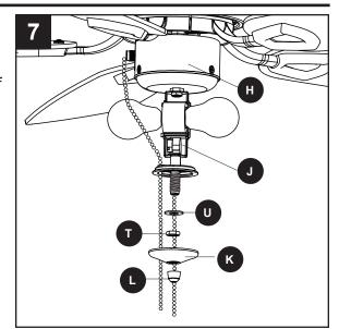
Feed the pull chain coming from the grommet in the light kit (J) through the off-center hole in the glass bowl (N). Feed the pull chain coming from the center of the light kit (J) through the center hole in the glass bowl (N).
