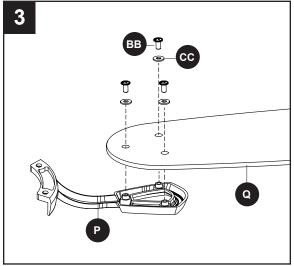
Install the blade arm (P) to the underside of the motor assembly (G) with motor screws (R) previously removed (Step 6, page 8). Tighten with Phillips screwdriver.
