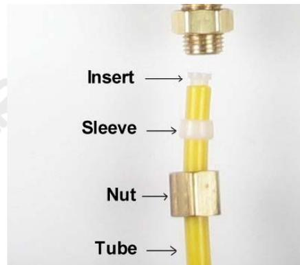
**Important!** Use plastic sleeve on the plastic tubing we provide. Do Not use metal sleeve on plastic tubing or the connection will leak!
