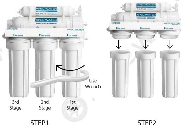
After taking the housing off, take out the dirty filters and put the new 3 pre-filters in. Remember, Stage 2 and Stage 3 are the same carbon filters.
