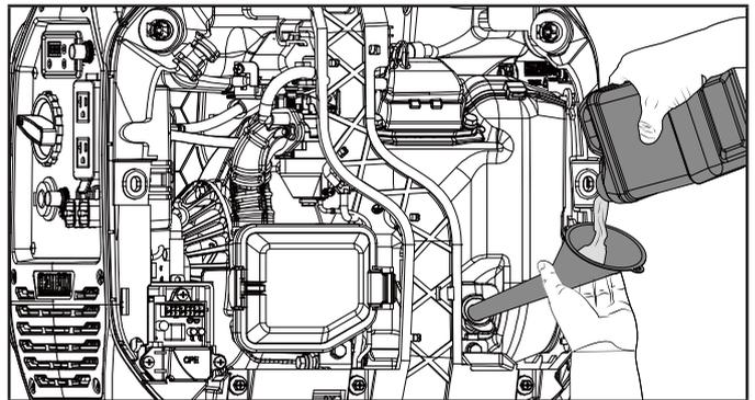
5. Check engine oil level before each use and add as needed.
