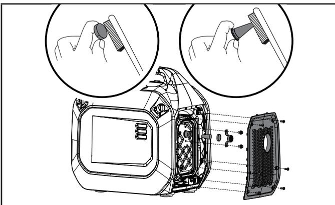
6. Replace the spark arrestor if it is damaged.
