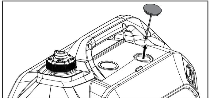
2. Remove the spark plug cable from the spark plug.
