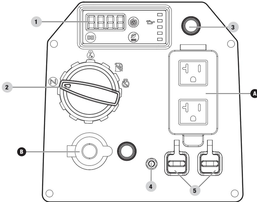
1. **Intelligauge with Power Meter and CO Shield®** – See *Intelligauge* section.
