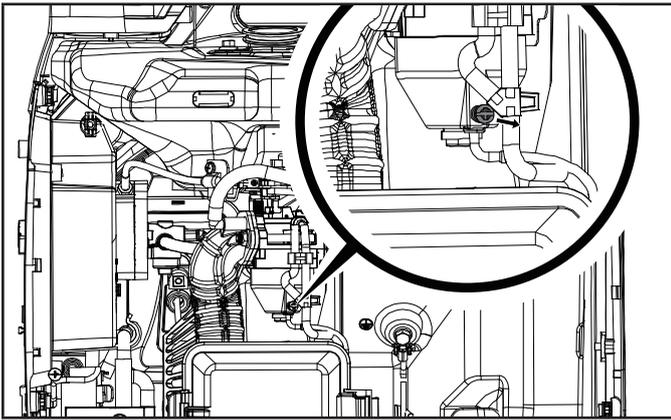
6. When gasoline stops flowing from the clear tube, rotate drain screw clockwise until tight. Properly dispose of the drained gasoline according to local regulations or guidelines.
