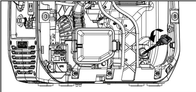
4. Tilt the generator on its side and allow the oil to drain completely.
