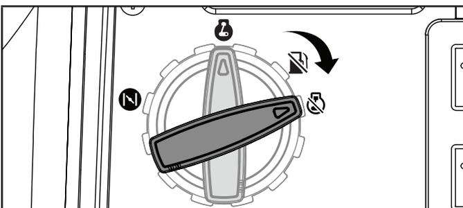
**Important:** Always ensure that the EZ Start dial and fuel vent lever are in the "OFF" position when the generator is not in use.
