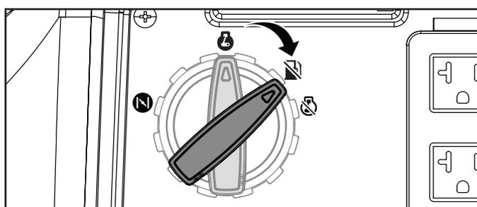
4. Let the engine run until fuel starvation has stopped the engine.
