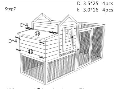
(1)Secure part (1) by using 4x screw(D).(2)Put on nesting box roof part (1), secure with 4x screw(E).
