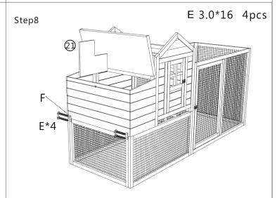
(1) Use 2x connectors part F to secure nesting box with bottom, use 4x screw(E) here.(2) Put in nesting box divider part 21
