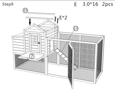
(1)Put on 2x perches part (1), and insert metal tray part (2)Secure ladder part (10), using 2x screw(E).
