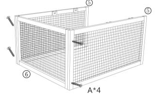
Connect 2x part 5 with part 6, secure with 4x screw(A).
