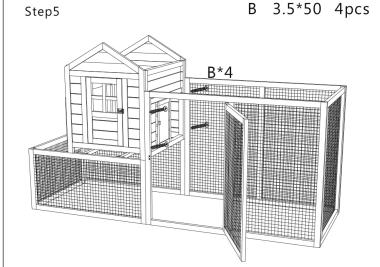
Put the part finished in step 4 above the part finished in step 3, secure with 4x screw(B) as shown.
