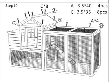
(1) Put on 2x roof part<sup>®</sup>, and roof cap part<sup>®</sup>, secure with 8x screw(C).
