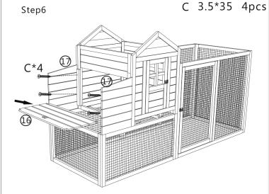
Secure 2x part①, each with 2x screw(C). Then put in nesting box floor part①
