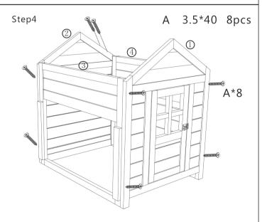
Connect part ①, ②, ③ and ④, and secure these four parts with 8x screw (A).
