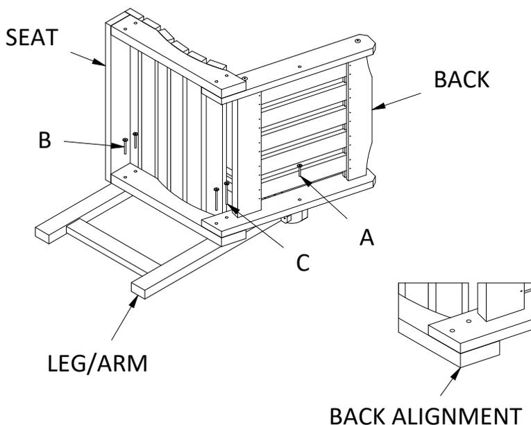
**1)** Attach Seat to Leg/Arm using (2) B bolts and (2) C bolts.
