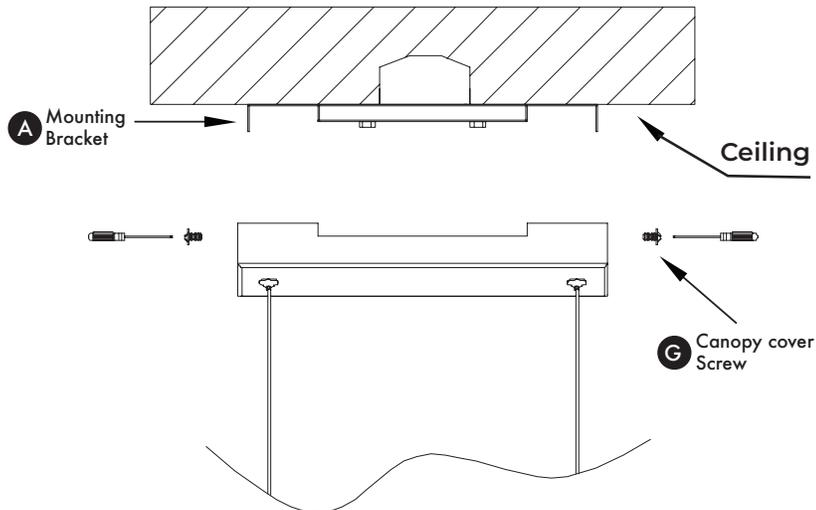
Secure canopy to mounting bracket (A) with canopy screws (G).
