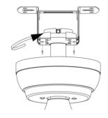
$\Box$  Place the canopy cover (if applicable) and rotate the canopy cover clockwise until it locks into position.
