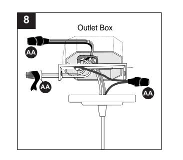
9. Carefully arrange excess wiring and wire connectors (AA) within canopy of fixture (A).
