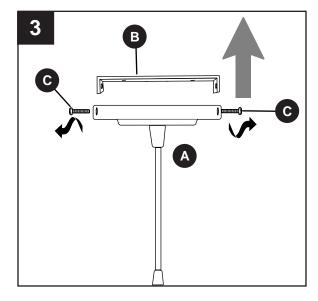
Attach mounting strap (B) to outlet box (not included) using the existing washers and outlet box screws or the machine screws (BB). NOTE: If the outlet box screws required for your outlet box are of a different size than the machine screws (BB), consult with a licensed electrician before proceeding.
