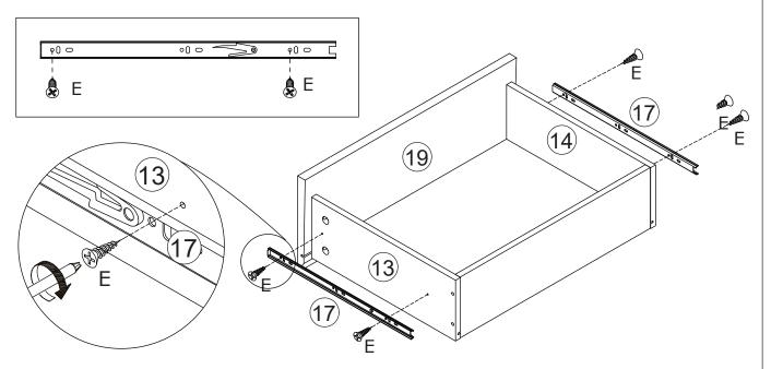
Fix slide rail 17 to part 13 and 14 using screw(E) as shown.
