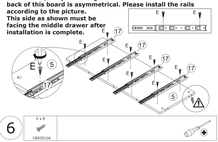
Fix slide rail 17 to the right of part 5 using screw(E) as shown.
