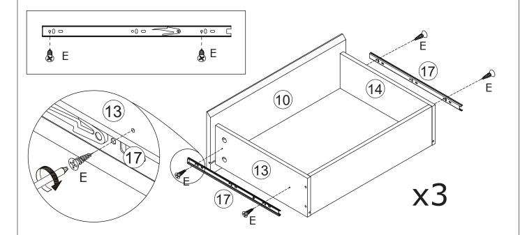
Fix slide rail 17 to part 13 and 14 using screw(E) as shown.
