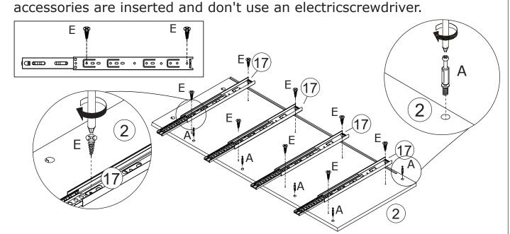
Insert quickfit screw(A) to part 3.Fix slide rail 17 to part 3 using screw(E) as shown.
