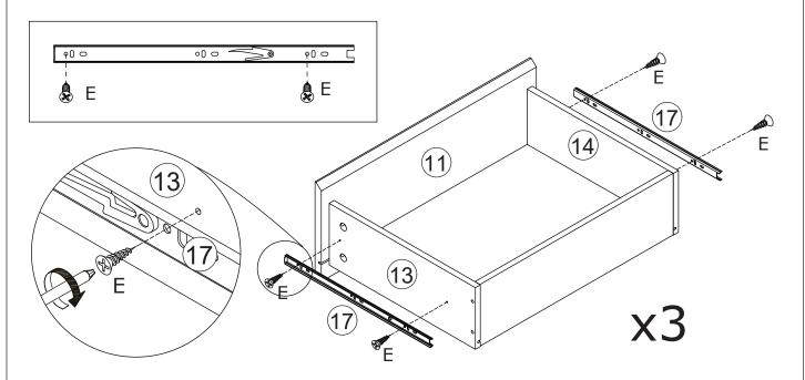
Fix slide rail 17 to part 13 and 14 using screw(E) as shown.  $\frac{24}{27}$
