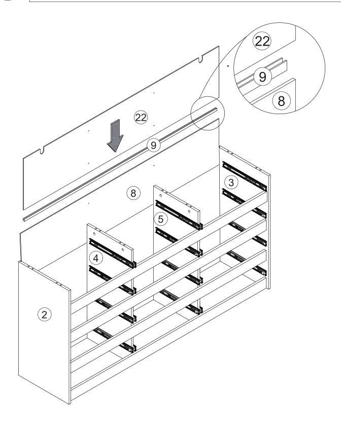
Connect part 8,22 with part 9 and insert into the available slots of part 2,3 and 7 as shown.
