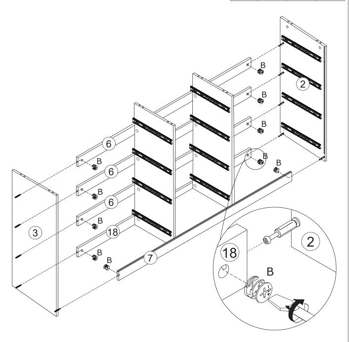
Attach part 2,3 to part 6,18 and 7, turn cam locks(B) clockwise to tighten as shown.
