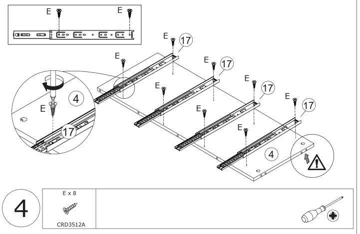
Fix slide rail 17 to the right of part 4 using screw(E) as shown.
