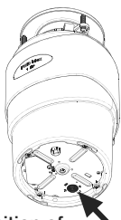
Position of the reset switch.
