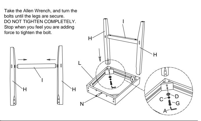
Put the Chair Back (M) on a smooth flat surface, attach the Seat Frame (L) to the Chair Back (M), using Bolt (E) or Bolt (F), Lock Washer (C) and Flat Washer (D) in both of hole of Seat Frame (L) and Chair Back (M) by Allen Wrench (A), but not too tight.
