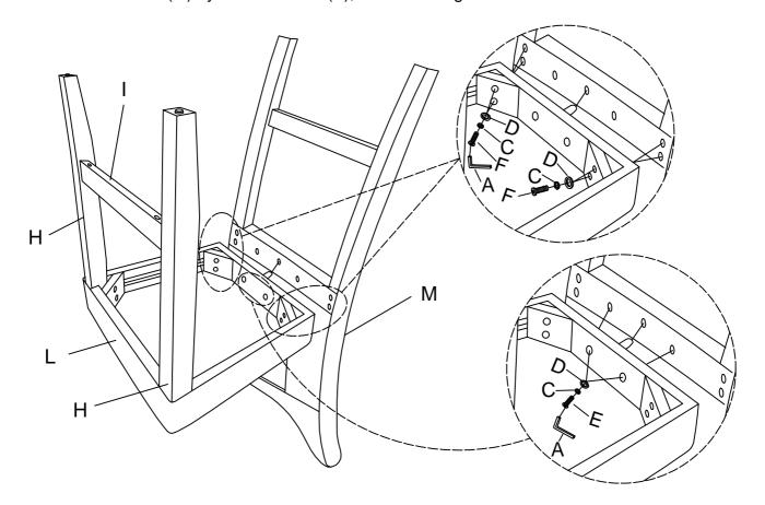
See drawing, assemble the Left Stretcher (J) and Right Stretcher (K) to Front Leg (H), and Chair Back (M), using Screw (B) and Glue (O) to secure all stretchers including Front Stretcher (I).
