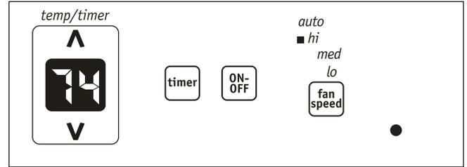
Note: Tap or hold either up (▲) or down (▼) button until the desired temperature is seen on the display. This temperature will be automatically maintained anywhere between 60 °F (16 °C) and 90 °F (32 °C). If you want the display to read the actual room temperature. See "To Operate on Fan Only" section on Page 6.
