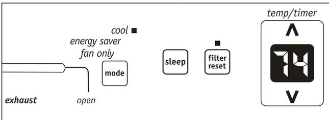
Note: This feature is a reminder to clean the Air Filter (See Care and Cleaning) for more efficient operation. The LED (light) will illuminate after 250 hours of operation. To reset after cleaning the filter, press the "Filter Reset" button and the light will go off.
