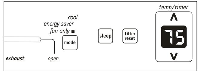
Note: Use this function only when cooling is not desired, such as for room air circulation or to exhaust stale air on some models. (Remember to open the vent during this function, but keep it closed during cooling for maximum cooling efficiency.) You can choose any fan speed you prefer. (Except "Auto Fan"). During this function, the display will show the actual room temperature, not the set temperature as in the cooling mode.
