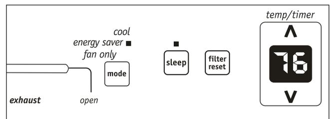
Note: In this mode the selected temperature will increase by 2 °F 30 minutes after the mode is selected. The temperature will then increase by another 2 °F after an additional 30 minutes. This new temperature will be maintained for 7 hours before it returns to the originally selected temperature. This ends the "Sleep" mode and the unit will continue to operate as originally programmed. The "Sleep" mode program can be cancelled at any time during operation by again pressing the "Sleep" button.
