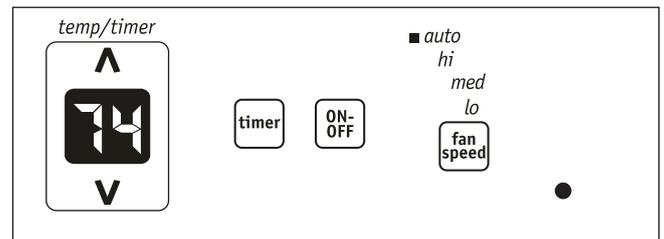
Note: Fan starts at High Speed and adjusts to a slower speeds the room temperature dictates. For example, if the room doesn't get too warm, it will stay at the slowest speed. If the room temperature rises quickly, such as a door being opened, it will automatically go to the highest speed. The fan speeds will re-adjust back to the slowest speed as the room returns to the original set temperature. Press either the fan slower or fan faster button to adjust the fan speed manually.
