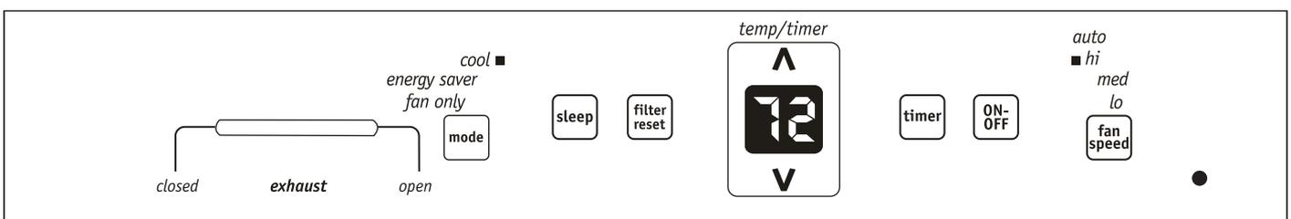
This Exhaust Control allows the air conditioner to either recirculate inside air (CLOSED) or exhaust air to the outside (OPEN). The CLOSED position is used when maximum cooling is desired. It may also be used for air recirculation without cooling when the air conditioner is set in any FAN position. The OPEN position removes stale air from the room and exhausts it to the outside. Fresh air is drawn in through normal passages in the home.
