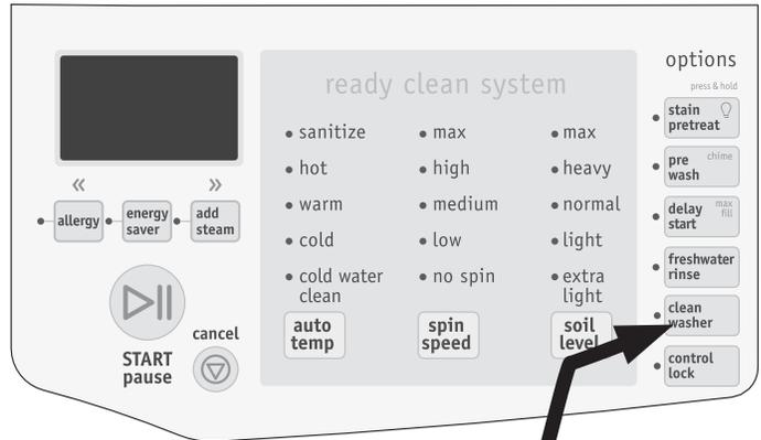
Turn cycle selector to **Rinse & Spin** and then press **Clean Washer** button to enter **Clean Washer** cycle.
