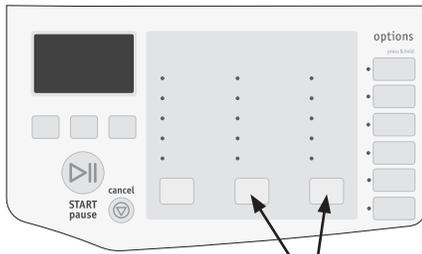
To return to factory settings, press these two buttons at the same time and hold until the signal sounds.
