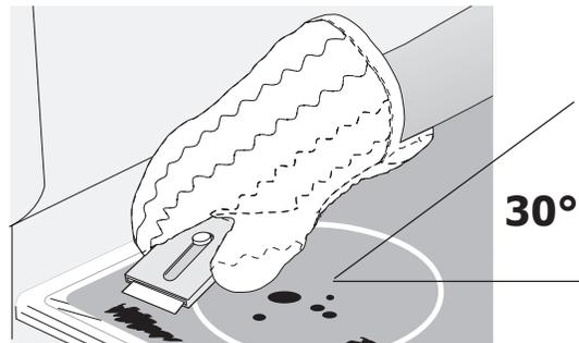
**Removing plastic or foods with a high sugar content:** These types of soils need be removed immediately if spilled or melted onto the ceramic cooktop surface. Permanent damage (such as pitting of the cooktop surface) may occur if not removed **immediately**. After turning the surface elements OFF, use a razor blade scraper or a metal spatula with a mitt and scrape the soil from the hot surface (as illustrated). Allow the cooktop to cool, and use the same method for heavy or burned on soils.
