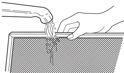
2. Soak the ventilation filters in hot water using a mild detergent. Rinse well and shake to dry or wash in a dishwasher. **Do not use ammonia. The aluminum on the filter will corrode and darken.**
