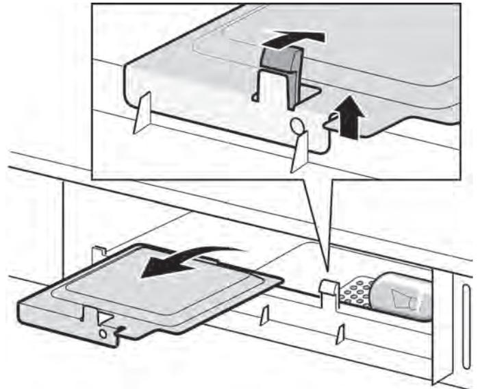
2. Remove old light bulb and replace only with equivalent 30 watt bulb available from parts distributor. Bulbs are also available at most hardware stores or lighting centers.
