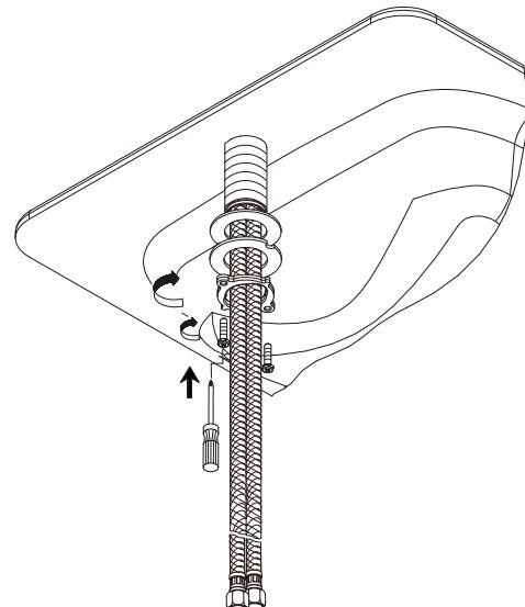
2. From underneath the sink, install washers and lock nut. Tighten the screws on the lock nut to secure the body.
