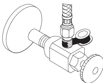
3. The supply hoses fit 3/8" supply valves. Apply pipe sealant tape to threads on valve before attaching the supply hose.
