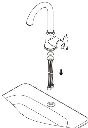
1. Insert faucet into 1 1/2" diameter mounting hole in deck from above.
