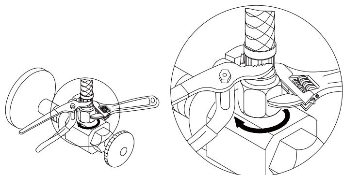
4. IMPORTANT! Tighten the hose onto water supply. Use two wrenches to avoid twisting hose when tightening.
