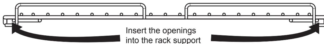
Insert the openings into the rack support
