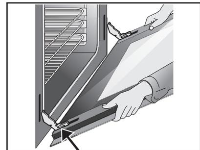
HINGE SLOT - Door removed from the appliance
