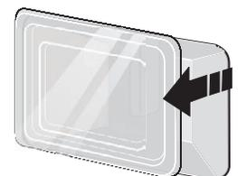
Lift backside of glass shield and remove it.
