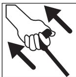
**12****Move the Choke to the OPEN Position**
