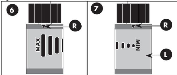
Adjust the pressure by rotating the adjustable pressure regulator (L) clockwise for higher pressure or counterclockwise for lower pressure, aligning the arrow with the desired pressure bar on the adjustable pressure regulator.
