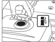
**IMPORTANT:** Ethanol Shield™ (sold separately) is a fuel stabilizer that helps eliminate and prevent ethanol related problems in power equipment. Follow the instructions on the container and add to the gasoline.
