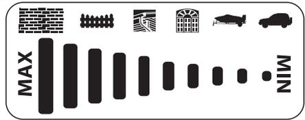
**NOTE:** To apply chemicals the black low pressure nozzle must be installed and the adjustable pressure regulator must be in the MAX pressure setting.
