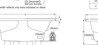
Letter Description **English** Metric L Outer Length 59 3/4" 1518 mm 41 3/4" W Outer Width 1060 mm Overall Height 26" 660 mm Α Overflow Height 20" 508 mm В Long Edge to Drain Center 11 3/4" 298 mm С Short Edge to Drain Center 32 1/2" 826 mm D Drain Shoe Length 6" 152 mm Ε Deck Height 2" 51 mm F Deck Width\* 3" 76 mm G Service Access Dimensions 305 mm x 457 mm 12" H x 18" L Floor Cut-out for Drain 17" x 4" 432 mm x 102 mm
