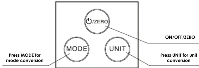
1. The On/Off-zero button is used to switch the scale on or off, and to reset the scale to 0.00 (Tare function).
