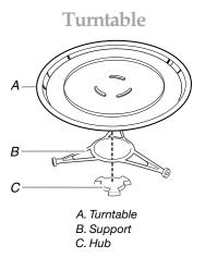
The turntable can rotate in either direction to help cook food more evenly. For best cooking results, do not operate the microwave oven without having the turntable in place. See "Assistance or Service" to reorder any of the parts.
