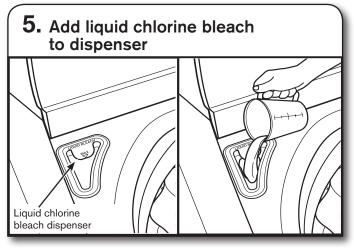
Do not overfill, dilute, or use more than 3/4 cup (180 mL). For maximum soil and stain removal, you may use the liquid chlorine bleach dispenser for liquid chlorine bleach or color-safe bleach.
