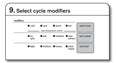
Once you select a cycle, the default settings for that cycle will be lit. Press the Modifier buttons to change the Wash Temp, Spin Speed, and Soil Level, if desired. Not all settings are available with all cycles.
