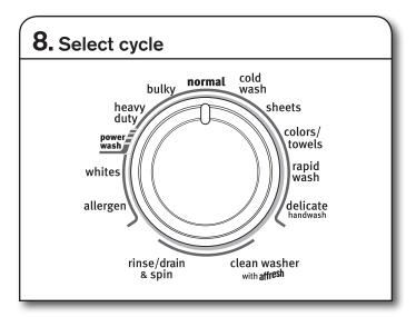
Turn cycle knob to choose your wash cycle. Estimated Time Remaining will light up with a cycle time. You may notice time adjusting during the cycle. This is normal.
