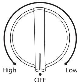
The control knobs can be set to anywhere between HIGH and LOW. Push in and turn to setting.
