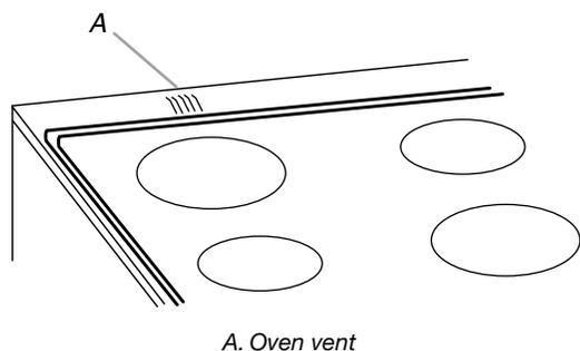
The oven vent releases hot air and moisture from the oven, and should not be blocked or covered. Blocking or covering the vent will cause poor air circulation, affecting cooking and cleaning results. Do not set plastics, paper or other items that could melt or burn near the oven vent.
